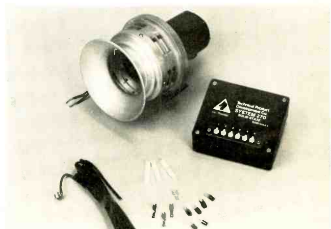
AUTOMOTIVE ALARM SYSTEM USES A SIREN to warn of tampering. The system shown is made by Technical Product Development Company.
