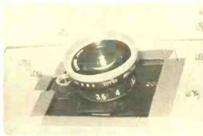
FIG. 3—CAMERA with lens adapter ring mounted on front panel of bracket.
